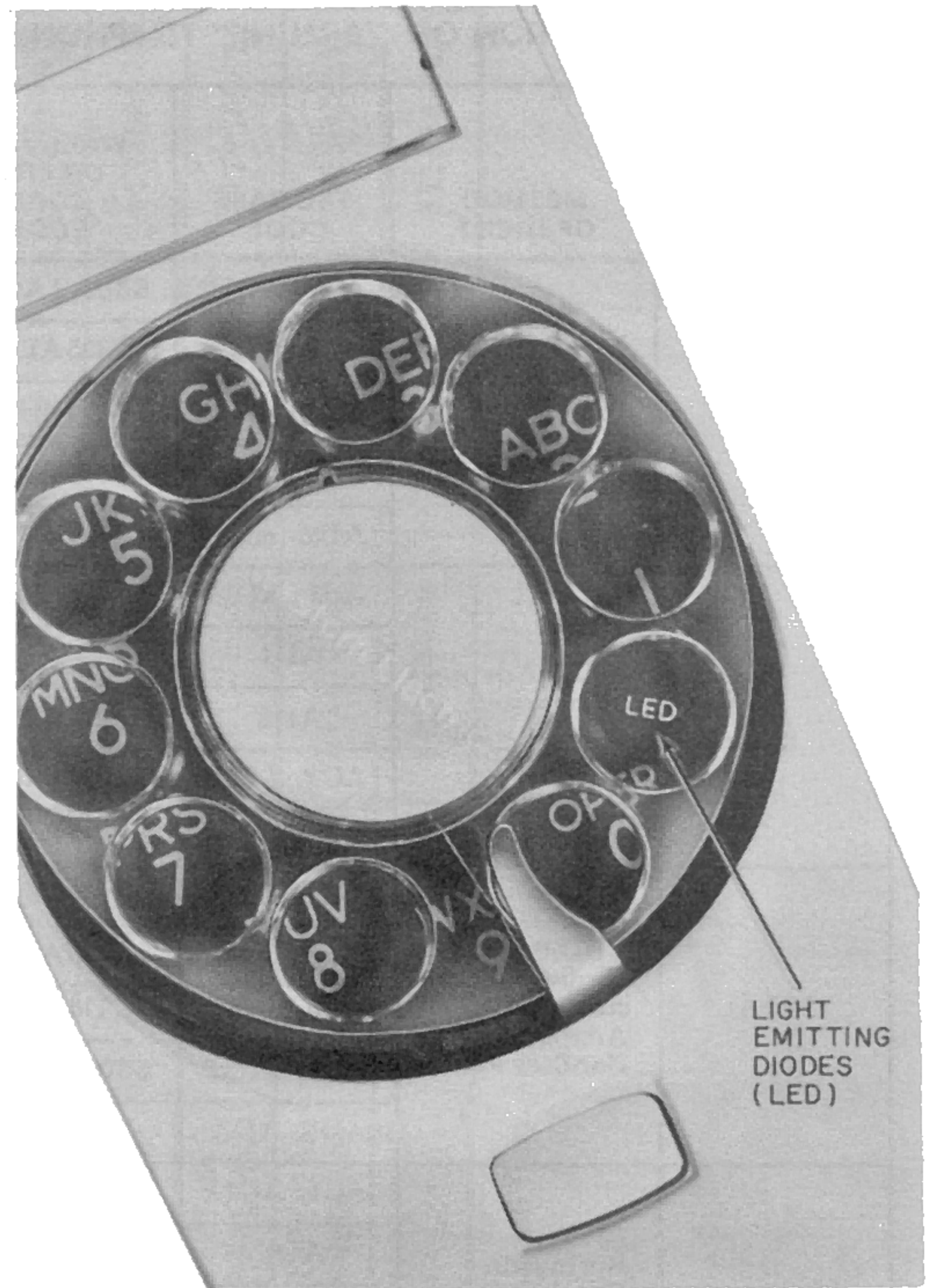
Fig. 5—220C, 220AL, and 226A Hand Telephone Set Identification Stamping (LED)
