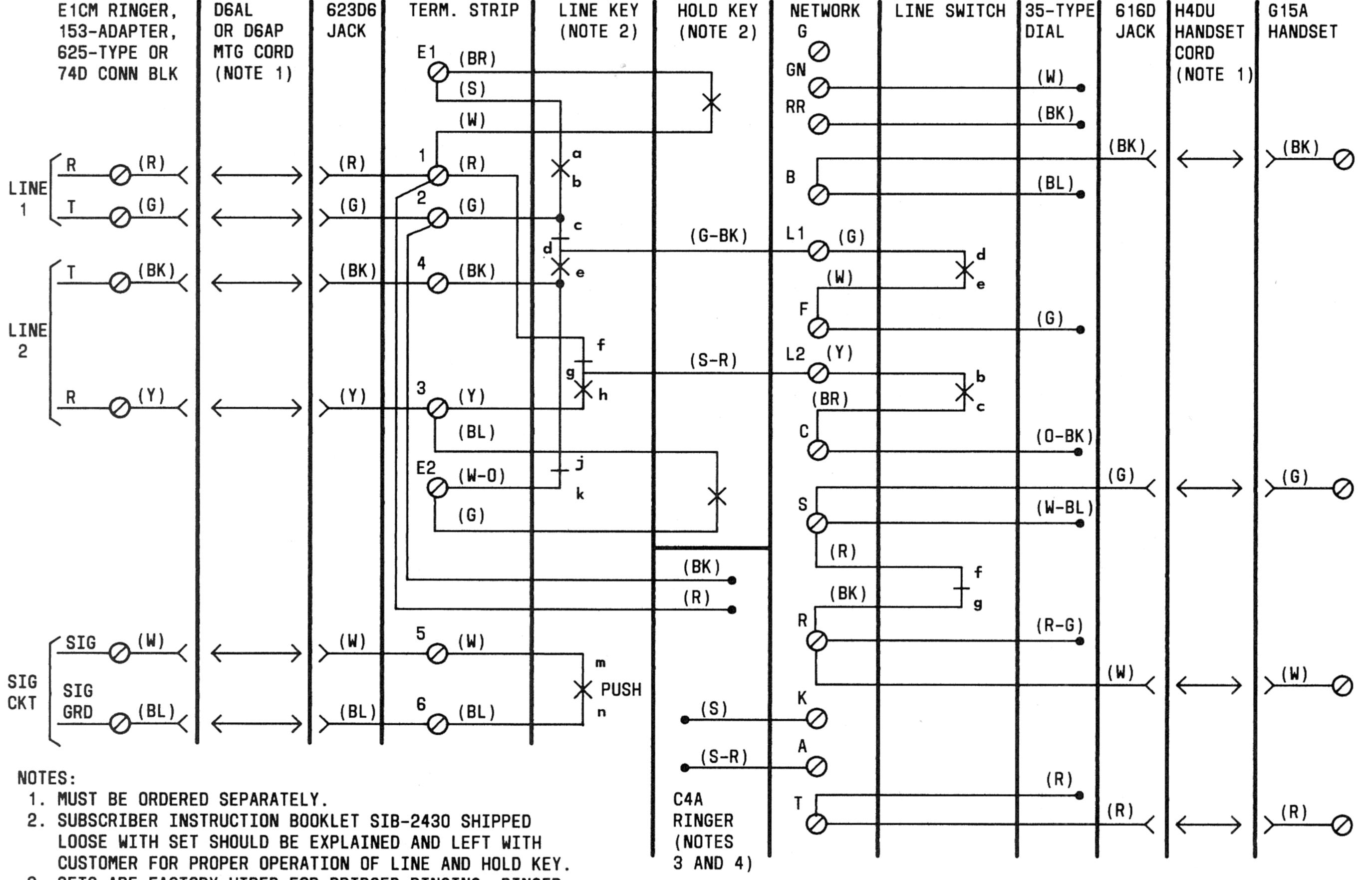
3. SETS ARE FACTORY WIRED FOR BRIDGED RINGING. RINGER CONNECTIONS PROVIDE FOR RINGING ON LINE 1. FOR RINGING ON LINE 2, CONNECT (R) AND (BK) RINGER LEADS TO TERMINALS 3 AND 4 RESPECTIVELY.
