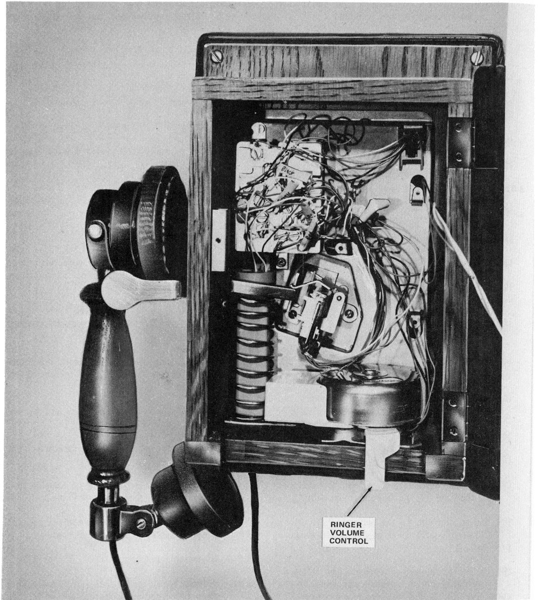
Fig. 3—951A1-03 Telephone Set With Front Panel Door Open
