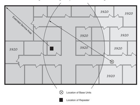
Figure 6: Using a Repeater to Extend Range
