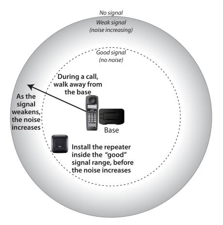
Figure 23: Mapping the Coverage Area of a Base Unit
