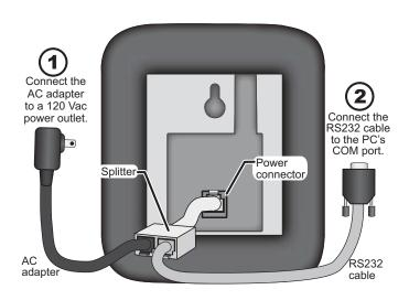
Figure 21: PC and Repeater Connections
