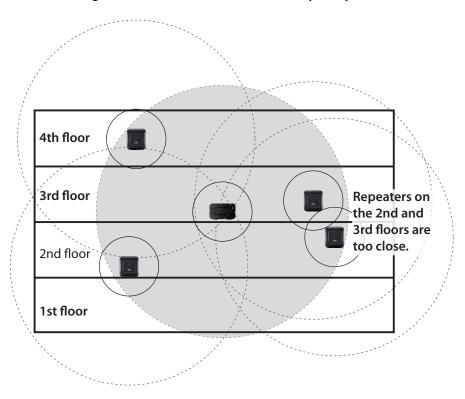
Figure 11: Incorrect Installation of Multiple Repeaters
