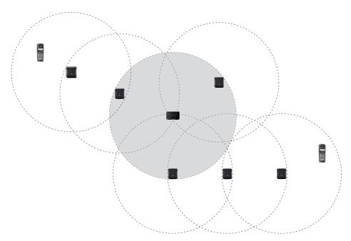
Figure 12: Combined Installation of Normal and Daisy-Chain Connections
