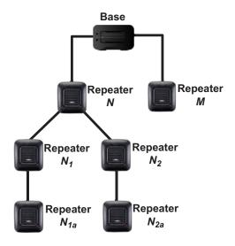
To install repeaters in a daisy-chain configuration, you must perform the following steps:
