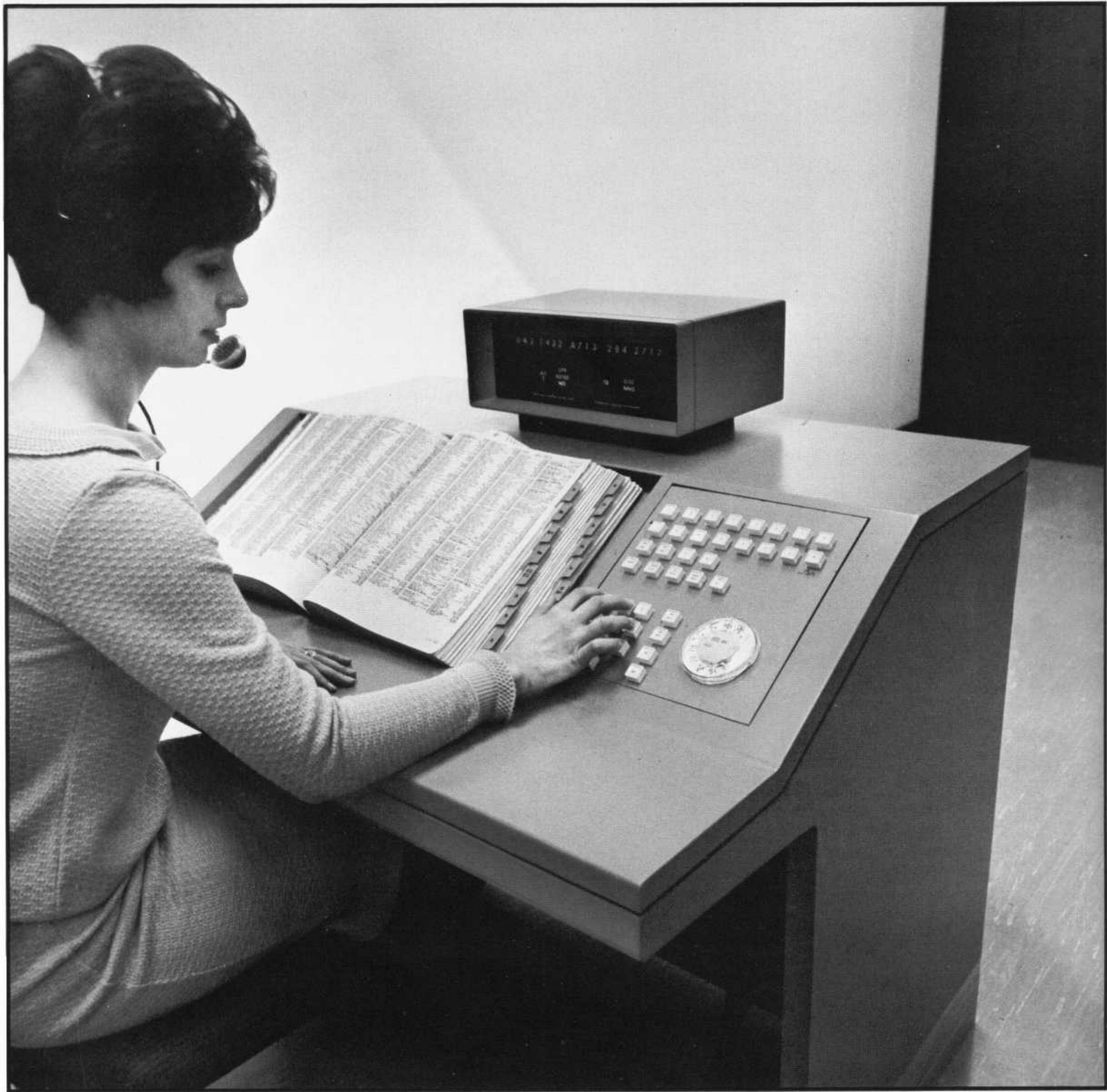
Mrs. G. Dane of the Holmdel laboratory demonstrates the use of the operator's console to be installed in a Centralized Intercept Bureau. This mockup model was constructed at BTL as part of the design project for the automatic intercept service.
