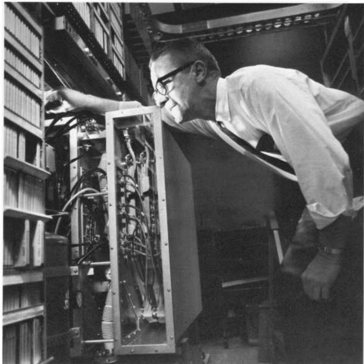
The author adjusts the pressure of the hydrogen atmosphere in which the disc files are kept. These files, which were purchased from an outside supplier, are part of the prototype Automatic Intercept System that was installed at the Holmdel laboratory.
