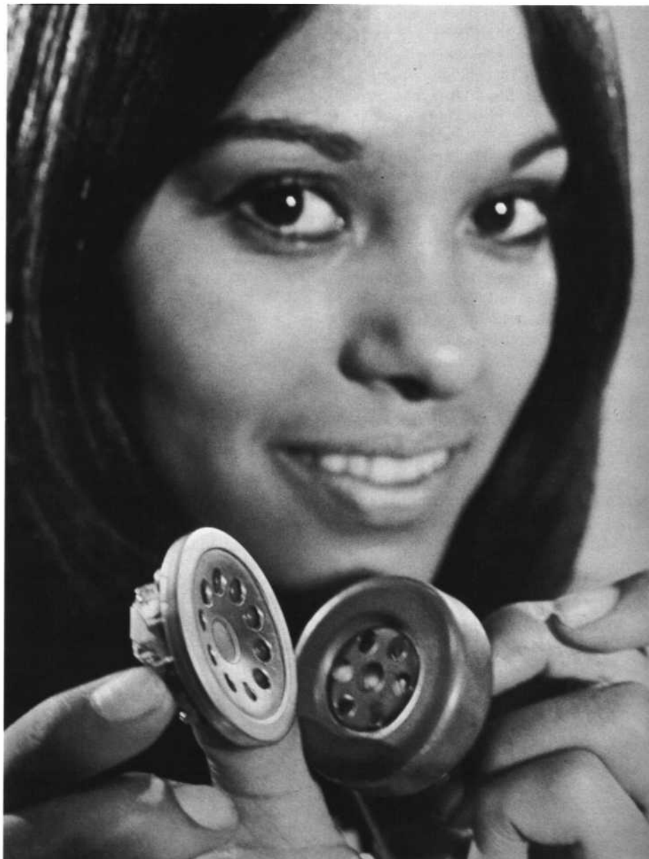
Bell Labs' Diane Johnathan holds a standard telephone receiver (right), and a smaller, unproved unit (left) which will eventually reap a savings of more than two hundred tons of strategic raw materials per year. The estimated savings in materials is based on an anticipated annual production rate of 10 million units. The new receiver will eventually be used in most Bell System telephone sets.
