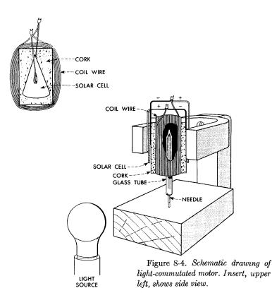
get in the space available on the cork for 30 ohms of wire. I used 350 turns of No. 31 Formex wire and the resistance was about right. This is not critical. To hold the windings in place, use household cement.
