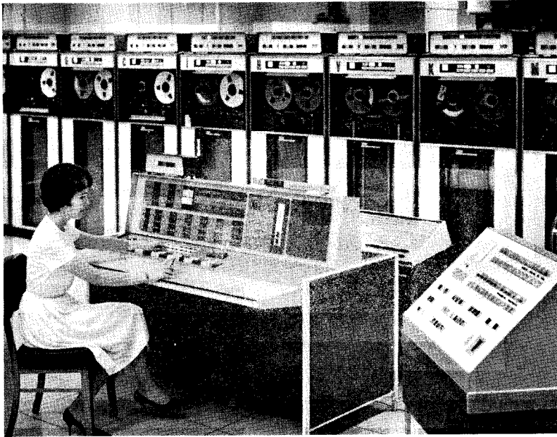
Fig. 1.3 Modern digital computers are used today to synthesize speech. Punched cards are fed to the computer; the computer reads and performs the instructions on these cards and produces a speech-like output on magnetic tape. The sounds are heard when the tape is played over a special tape recorder.
