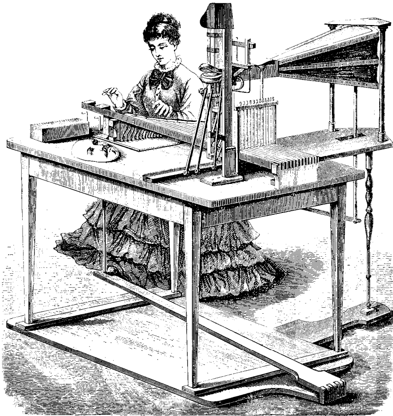
Fig. 1.1 Faber's talking machine, developed around 1850, could hold a conversation in normal speech. A foot-operated lever pumped the bellows at the top right. Air streaming from the bellows activated a vibrating reed whose buzz was modified by the resonances of the tubes on the operator's left side and by the lip-like opening directly above the tubes. The keyboard played by the young lady determined which resonant tubes were in use. The mask face-up on the front of the machine was included to complete the illusion.
