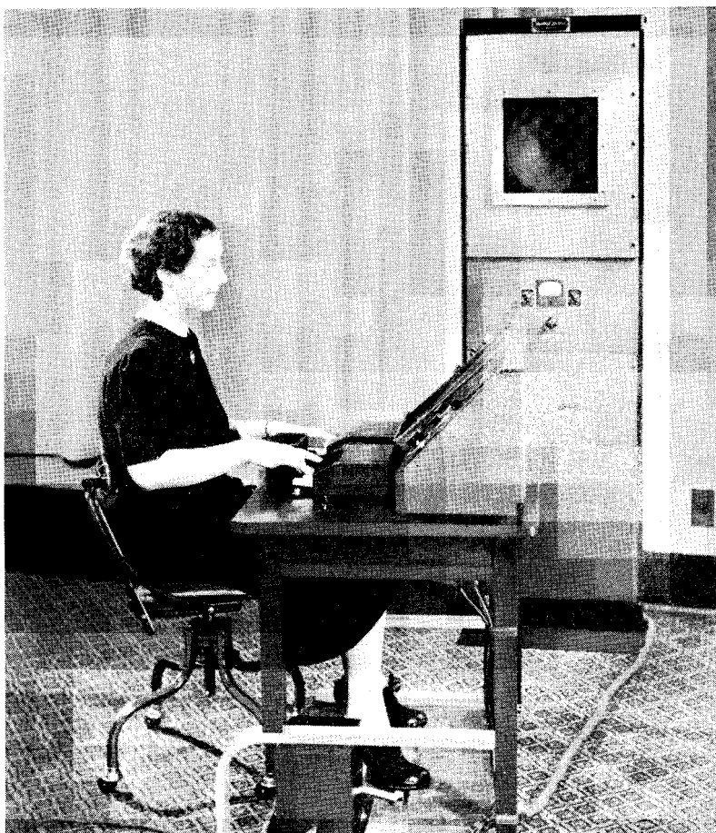
Fig. 1.2 The Voder, an electronic synthesizer, was exhibited at the 1939 World's Fair in New York. The young lady in the photograph could carry on a conversation by pressing keys; 13 keys controlled the speech sound produced and another key controlled volume. Three other keys were used to make the "stop" consonants. A foot-operated pedal gave rising and falling inflections.
