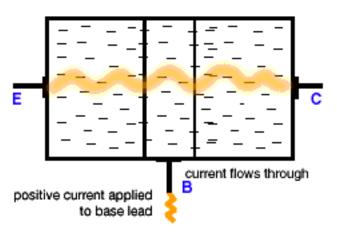
This animation shows the transistor effect as the transistor is made to alter its state from a starting condition of insulation (switched 'off', no current flow) to a final condition of conductivity (switched 'on', full current flow).
