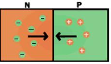
tendencies in the "p" and "n" regions and could reproduce them at will. With the discovery of the P-N junction and the ability to control its properties, the fundamental ground work was laid for the invention of the transistor. This Bell Labs discovery was instrumental in the development of all semiconductor devices to come.
