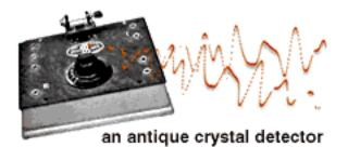
Seeking a new method of detection, the scientists reverted to the antiquated "cat's whiskers" detector, which was based on a crystal. Not only did it work effectively, it also set them on the path of exploring the particular properties of the most reliable semiconductor material: silicon.
