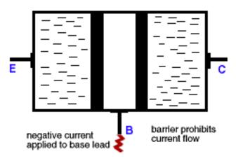
This shows the transistor effect as the transistor is made to alter its state from a starting condition of conductivity (switched 'on', full current flow) to a final condition of insulation (switched 'off', no current flow).
